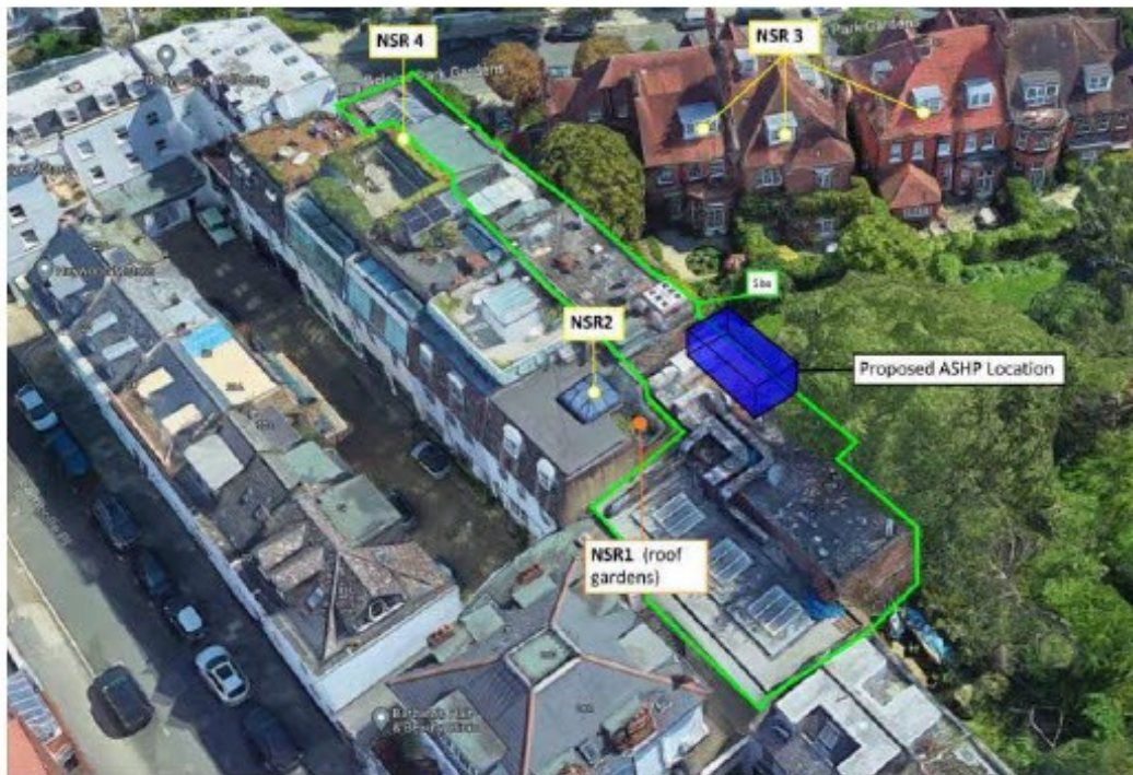
Figure 4: Proposed location of the 2No. ASHPs, and the nearest noise-sensitive receptors (NSRs)
